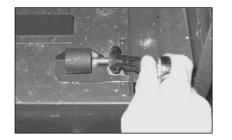
**Figure 6.5** Replace orifice with the proper size as indicated below for your gas type and venting. Re-install burner. Slide burner neck into shutter and over orifice. Re-install burner pan locators on left and right side of the burner. Secure with one screw to each side.
